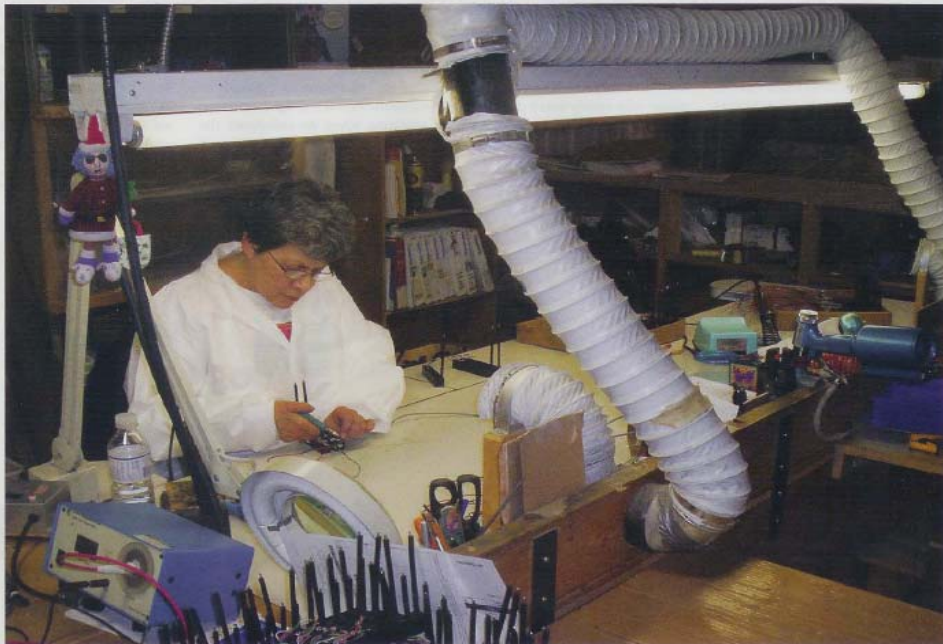
Valerie Barr tests high-voltage power supplies before they go into polarized-media electronic air cleaners.
