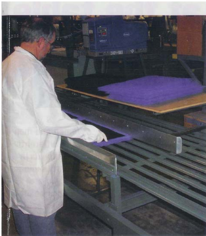
Ray Sample fabricates polarized-media, shown with the carbon center screens used in the air cleaner media.
