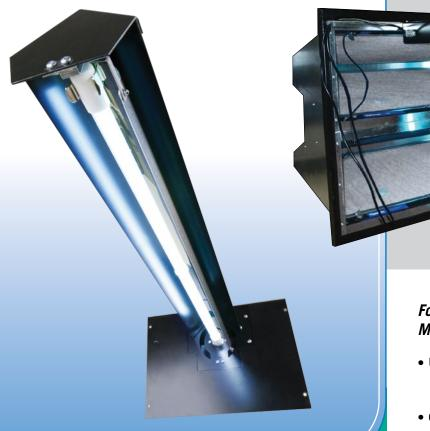
The Dynamic Sterile Sweep features a germicidal lamp with an oscillating reflector that kills pathogens collected by the Dynamic Air Cleaners as it slowly oscillates over the filter media surface area. The parabolic reflector provides additional concentration of UVC light. Sterile Sweep high output UVC systems offer the most effective means of controlling airborne pathogens and viruses including COVID-19.
